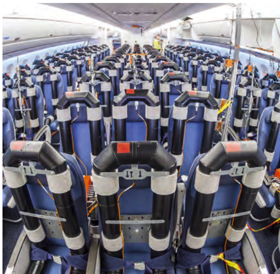
LEFT: THE TESTS CARRIED OUT IN THE CABIN OF MSN2, AIRBUS'S A350 TEST AIRCRAFT, INCLUDED INTENSIVE AIR QUALITY EVALUATIONS
