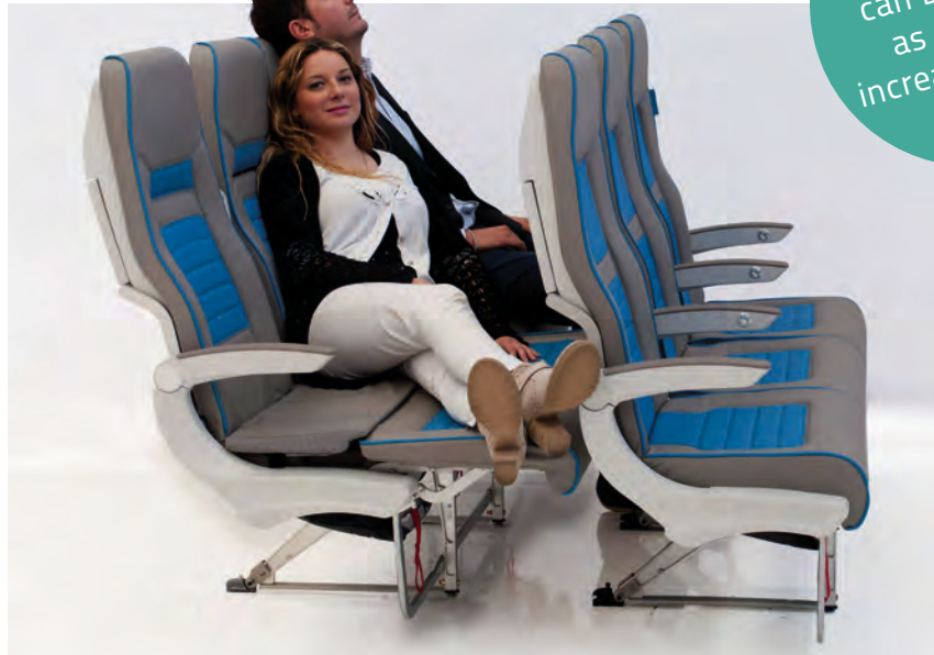
ABOVE: THE Y-BED TURNS A SEAT QUAD OR TRIPLE INTO A COMPANION TRAVEL SPACE LEFT: SKY-NAP KEEPS THE HEAD IN PLACE TO HELP PASSENGERS SLEEP
