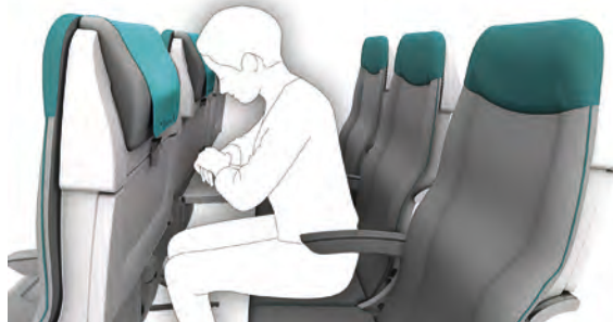
ABOVE: THE Y-BED TURNS A SEAT QUAD OR TRIPLE INTO A COMPANION TRAVEL SPACE LEFT: SKY-NAP KEEPS THE HEAD IN PLACE TO HELP PASSENGERS SLEEP
